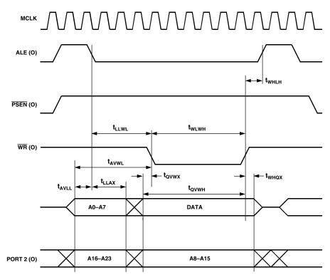
Figure 53. External Data Memory Write Cycle
